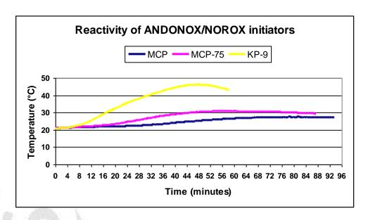
A reactivity test with an epoxy vinyl ester gave the following results:
